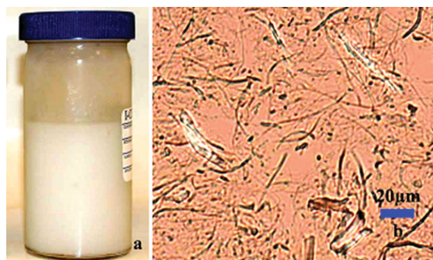
Figure 5 Suspension (a) and PLM image (b) of TC40 treated by HPH after HIUS 30-min treatment. [Color figure can be viewed in the online issue, which is available at www.interscience.wiley.com .]
